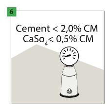
In the case of the cement grout, the moisture content in the substrate must be lower than 2.0%, and in the case of the anhydrite grout, it must be lower than 0.5%. In the case of installation with the underfloor heating, the abovementioned values must be 1.8% and 0.3% respectively.
