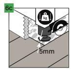
In the case of any heavy objects placed on the floor (such as kitchen furniture, kitchen island, built-in wardrobes and other furniture permanently attached to the wall), 5mm expansion joints should be left around them. We recommend the following ways to preserve expansion joint spaces:
