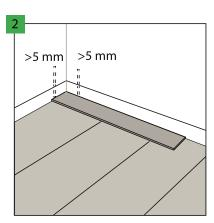
Leave 5 mm of perimeter space at the walls to allow the floor expansion. The maximum surface which can be laid without additional expansion joints is 200 m². Above this surface, apply an additional expansion joint and enlarge all the expansion joints up to 10 mm. The maximum length of the floor surface in one direction, which can be laid without additional expansion joints is 20 m. Above this length, apply an additional expansion joint and enlarge all the expansion joints up to 10 mm.
