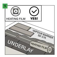
Installation on a heating foil is also allowed, provided that an appropriate underlay for the heating film and a vapor barrier foil SD ≥75 are used. The entire system consists of a vapor barrier foil laid directly on the substrate, then an appropriate underlay (min. 400 kPa, the recommended thickness of the underlay is 5 mm), a heating foil, a vapor barrier foil and the floor.
