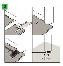
At the doors, it is recommended to undercut the profiles of door frames and leave free space over the installed panel so as not to limit its possible movement.
